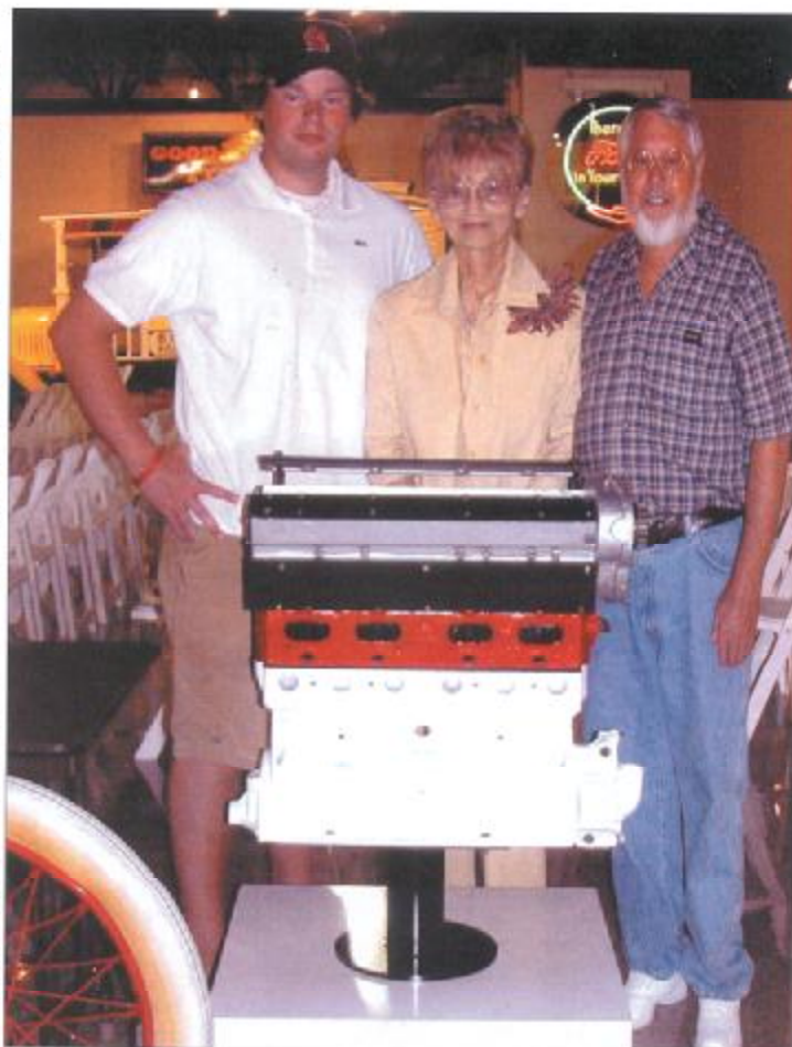
Betty Kerbs Abel, grandson Josh, and Fred Houston with what is believed to be the first DOHC Model T engine ever raced (during 1921 season). This dual overhead cam Craig-Hunt head was developed by Leonard Kerbs and his machinist, John Schoeber, three years before the DO Fronty. This engine is now part of the Smith Collection.
