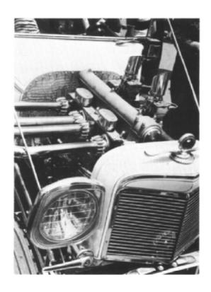
The engine is connected to a '39 Ford transmission which, according to Joe, is to be replaced with something stronger because he has gone through seven of them so far. The frame is of his own design and weighs only 68 pounds. The rear end is made of Model A housings, and runs Model A gears, but the other parts are of his own making. Axles are from a '26 Hudson.
