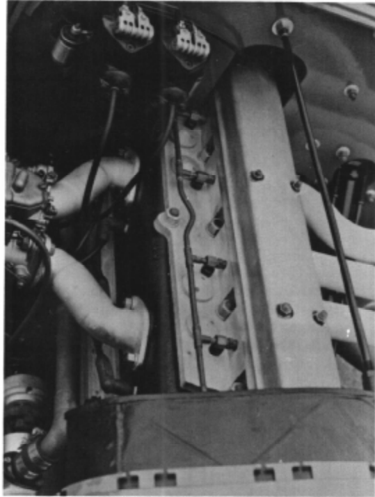
Top view of the engine shows the careful workmanship, typical of the whole car. The small pipe supplies oil to the camshaft bearings. The four plugs on the top plate cover the head bolts which thread into the old T valve guides.
