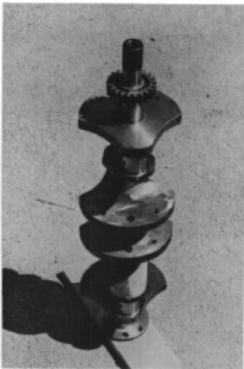
Counterweighted crankshaft is built up from 1928 Model A Ford. Shaft was shortened to fit T block by compressing the rear main and then grinding it back to size. Counterweights are steel and welded in place.
