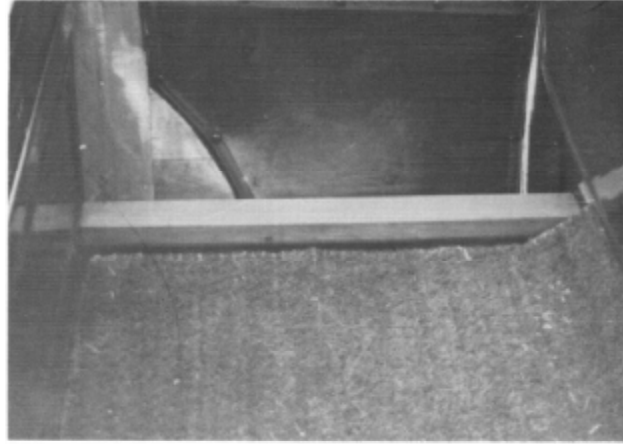
Early production Touring body sills (above) proved inadequate; were increased in size and a steel reinforcing plate added (below).
