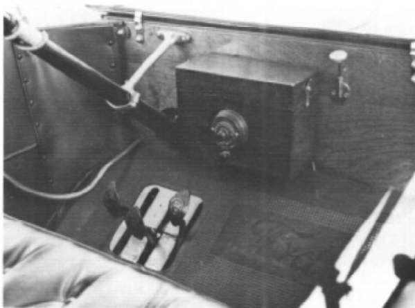
Coil box on our feature car is Heinze (left). K-W units were also used (right). This was the last year in which the wooden boxes were used.
