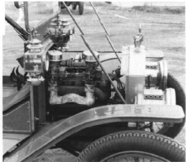
Orville Enyeart is still at it. Here s his 1909 with a hot engine. The car made the hill in 11.60. Aside from the dual carburetors, the engine has a Model A crank.
