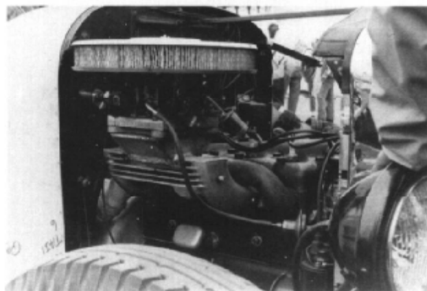
This speedster, owned by R. D Antonio, uses a stock T crank and head, but a four-barrel carburetor! The combination apparently works; the car made the hill in 11.108 seconds.
