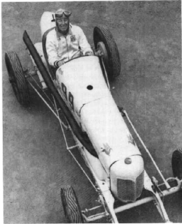
The Hooker Special, owned by Lindley Bothwell (in the car). The car was originally sponsored by Harry Hooker, an Arizona rancher, and held a number of dirt track records in the late twenties. The engine was (is) Model T with an overhead cam head designed by Harry Miller.
