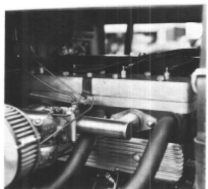
An interesting homemade flathead was entered by Ray Brindos (Car 41). The head is fabricated from two pieces of aluminum, with the water jackets and combustion chambers being milled in both pieces before they are joined.
