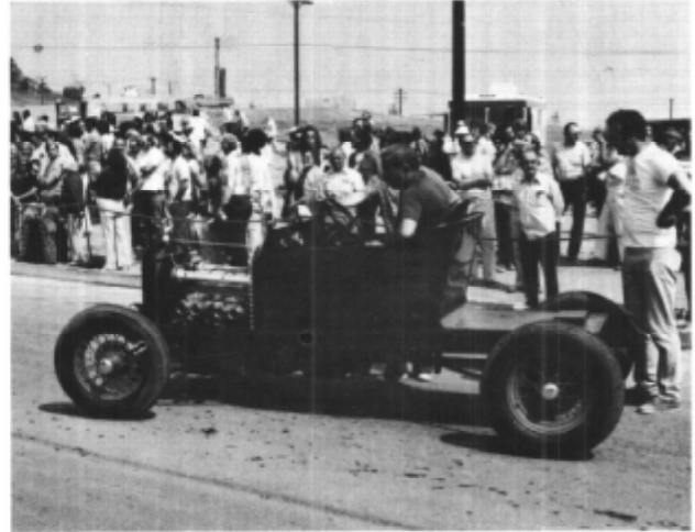
The second hottest car on the Hill was this Gemsa dual overhead cam roadster owned by LaRue Thomas. While this engine had more power than Hank Beckers speedster, the weight of the roadster body held it back (but by less than a second). The car has an automatic transmission; the ranges of which are selected by moving the 'brake lever.
