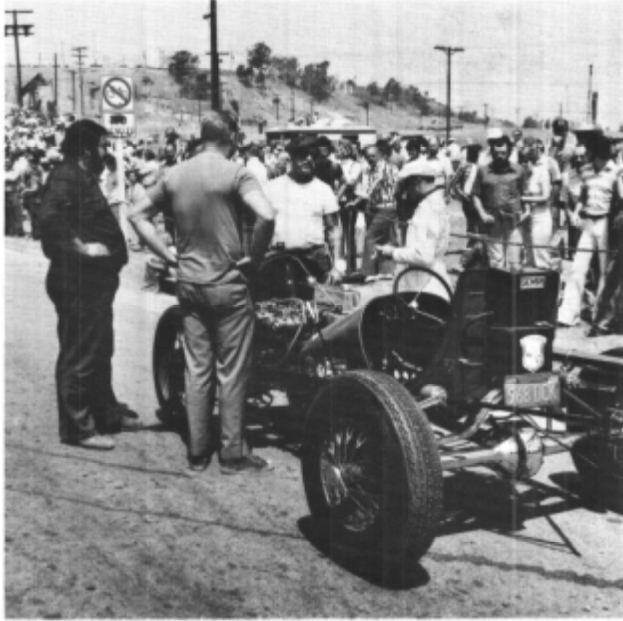
Hank Becker's Gemsa powered speedster. Hill climb rules call for a T block and a T frame in the Unlimited Class and that's about all there is "T" about the car. Note the many holes drilled in the frame, front axle, etc. to cut down the weight.
