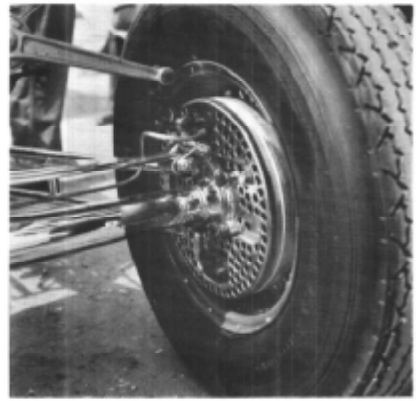
Hank Becker's Gemsa powered speedster. Hill climb rules call for a T block and a T frame in the Unlimited Class and that's about all there is "T" about the car. Note the many holes drilled in the frame, front axle, etc. to cut down the weight.
