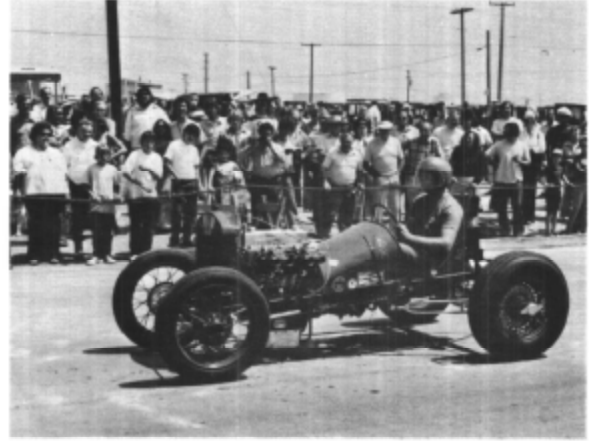
Hank Becker's Gemsa powered speedster. Hill climb rules call for a T block and a T frame in the Unlimited Class and that's about all there is "T" about the car. Note the many holes drilled in the frame, front axle, etc. to cut down the weight.
