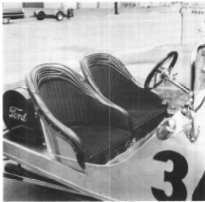
Pat Church's speedster has a beautiful newly-made aluminum body, done by a real professional. The engine and running gear are essentially stock.
