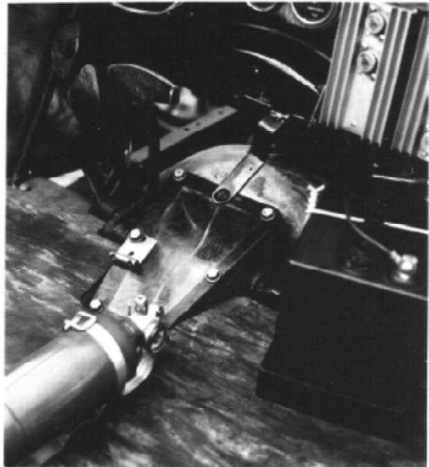
Have you ever wondered if the oil really did flow in the T engine? This owner apparently did and to make sure he put a clear plastic cover on the transmission. One thing for sure; you can watch the bands wear out.
