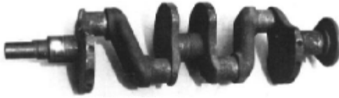
Model C Ford crankshaft. The best of all the stock Ford cranks. A bit difficult to modify to fit a T block unless it is to be an overhead cam conversion, but it can be put in if you work at it. The main problem is that the counterweights hit the camshaft in the T block.
