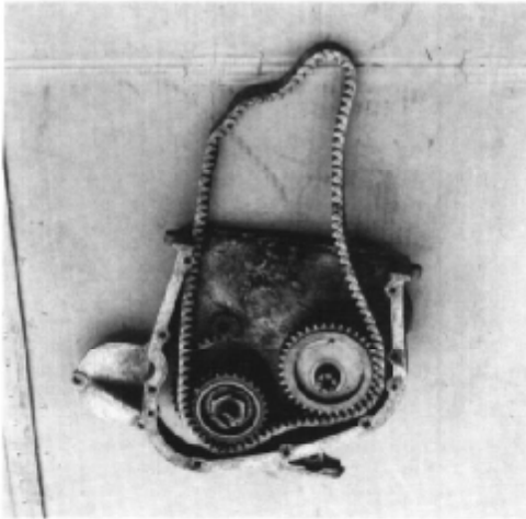
Fronty lower chaincase with the cover removed, showing the chain drive (silent chain) with idler and tension sprocket and the drive sprocket. There were two types of chain drive, the silent chain and the triple-roller chain. The silent chain is the earlier.
