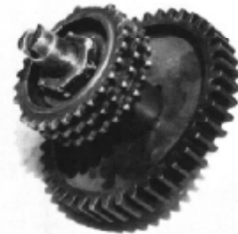
The cam stub shaft with the steel timing gear and the lower sprocket for the triple-roller timing chain. The slot in the front end of the shaft drives the oil pump.
