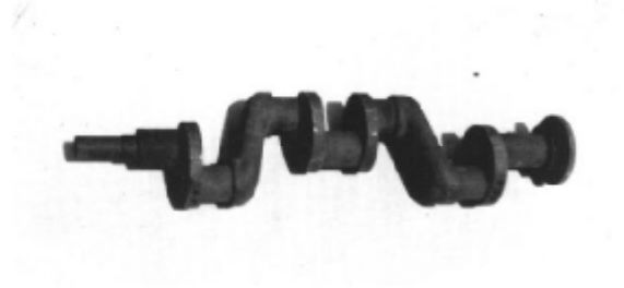
The stock Model B Ford crankshaft. These were used in racing T engines during the Thirties.
