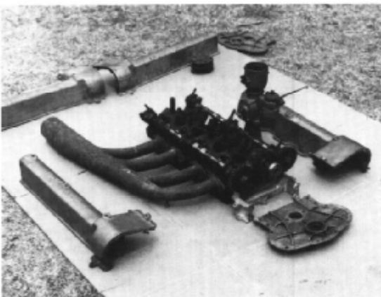
A complete factory D.O. Fronty with cam covers removed. The manifolds and carburetor are factory parts and very rare.
