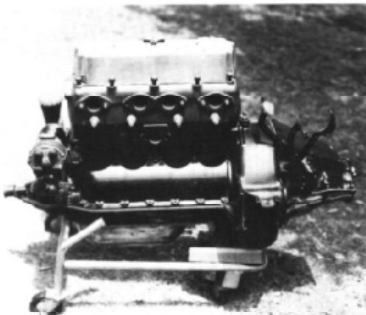
Intake side of the Model BB, showing the Reed carburetors, one set of spark plugs, aluminum oil sump for four-dip pan (original) and original aluminum side covers.
