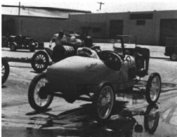
Few cars with original or original-like accessory bodies are seen these days. This "Faultless bodied speedster is owned by George Azcvedo. The car also has a Ruckstell axle, magneto ignition and dual carburetors – and Buffalo wire wheels.
