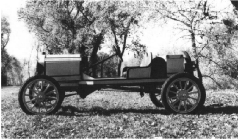
Rakish, low steering with twin bucket seats, Dodge gas tank, and a tool box.
