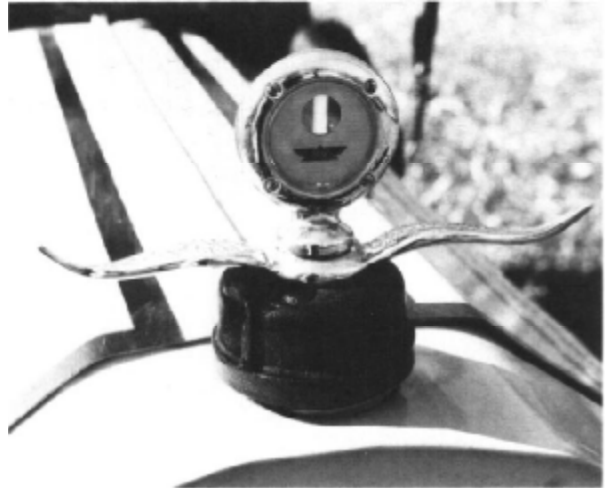
Three-inch pipe cap radiator cap with its moto-meter.
