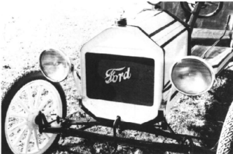
The mid-twenties Chevrolet headlights, $50 special radiator shell and the lengthened hood.
