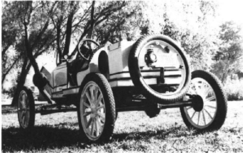
Rakish, low steering with twin bucket seats, Dodge gas tank, and a tool box.
