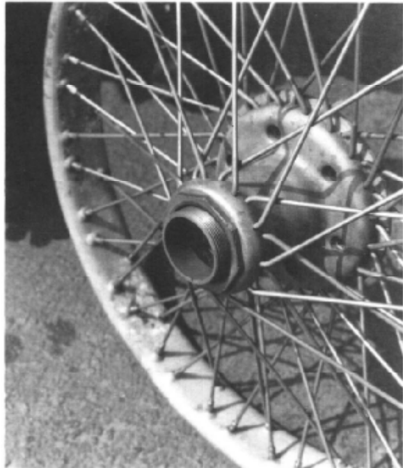
Pasco 30 x 3½ wire wheel and hub with only the wheel retaining nut installed.
