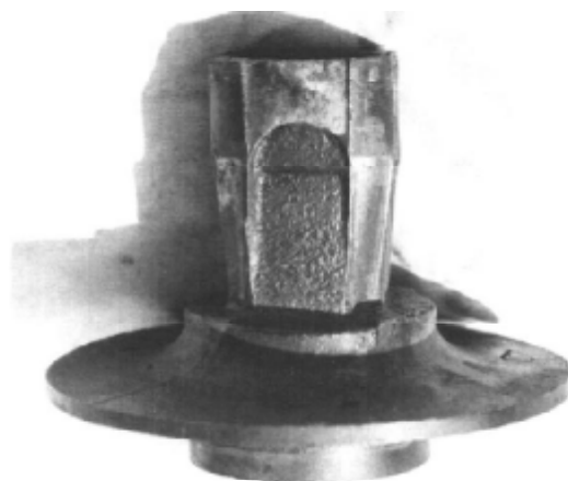
Side view of the Stewart front hub showing the odd square shape with flats milled for the retaining wedges on the hub cap.
