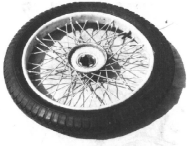
Rear of Stewart wheel showing the distinctive cross-shaped center hole.
