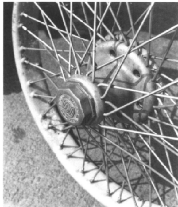
Pasco retaining nut and hub cap which locks it in place.
