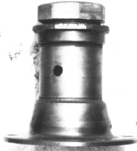
Pasco wheel with hub cap installed over the retaining nut.
