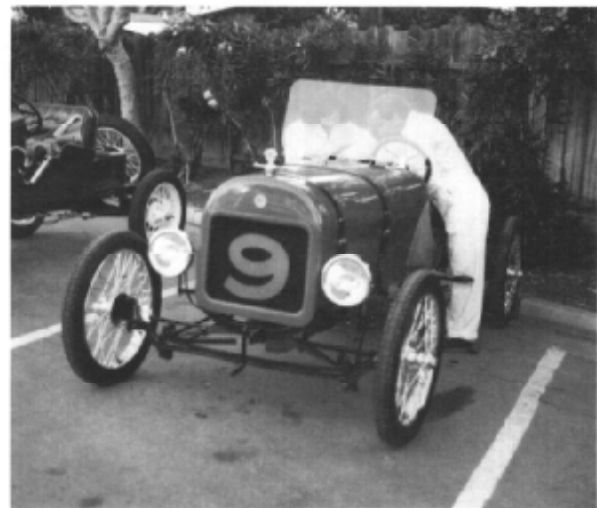
1912 speedster with stock engine, Winfield carburetor and a Bosch distributor. Driver is Joel Pencer; mechanic, Scott Pencer.
