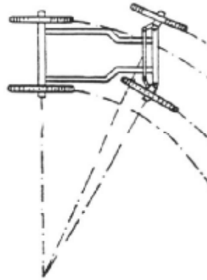
Fig. 2. Showing how the front wheels of an automobile give the direction the car runs.
