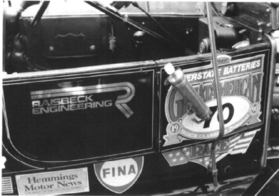
Left: An external hand pump was operated by the navigator to pressurize the gas tank to overcome vapor locks in the mountains. Below: The gas tank modifications are visible at the top of the tank.
