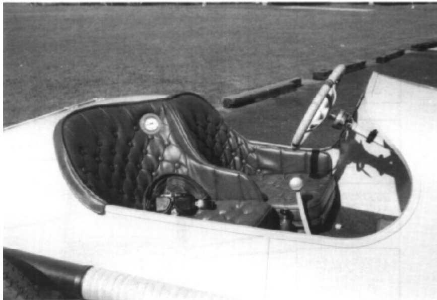
Above: The upholstery is diamond tufted leatherette. The diamond pattern was copied from an original picture. The fuel pressure gauge is mounted on the passenger's seatback. It is mounted here because pre-1920 bodies had no dashboard. It appears that the mounting location stayed the same on later bodies equipped with dashboards.
