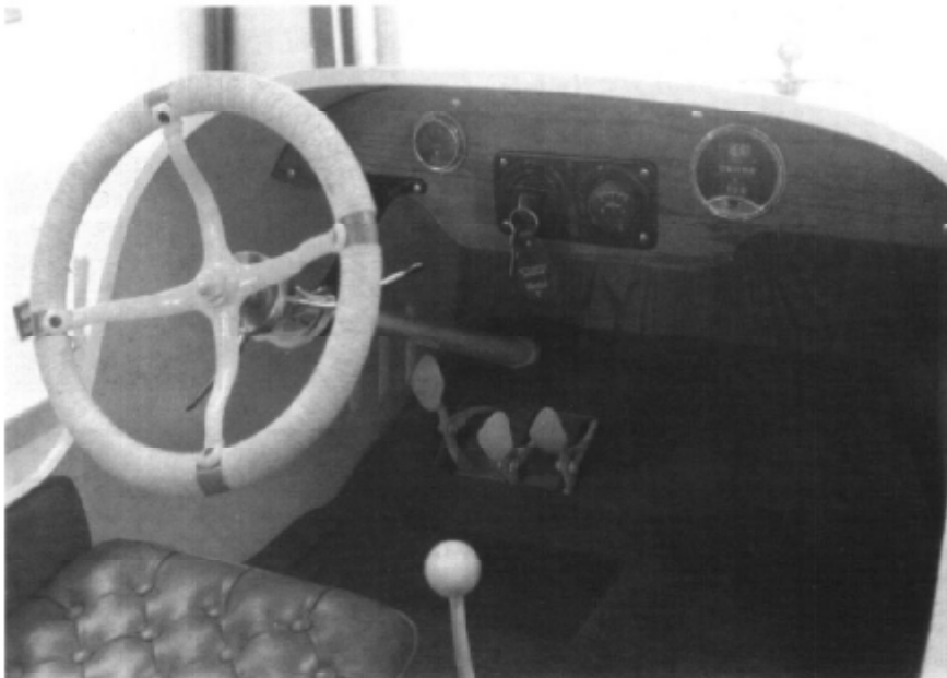
Below: The steering wheel has been reversed on the column to provide hand clearance around the cowl. The foot pedals are mounted on a common cross shaft 6 inches behind the original pedals. Rods with clevises run from the new pedals forward to the original pedals. The heads of the original pedals have been removed in order to clear the floorboards. A special bracket which came with the body braces the steering column. On the dash an oil pressure gauge, ignition switch/lampmeter, and AC speedometer are mounted.
