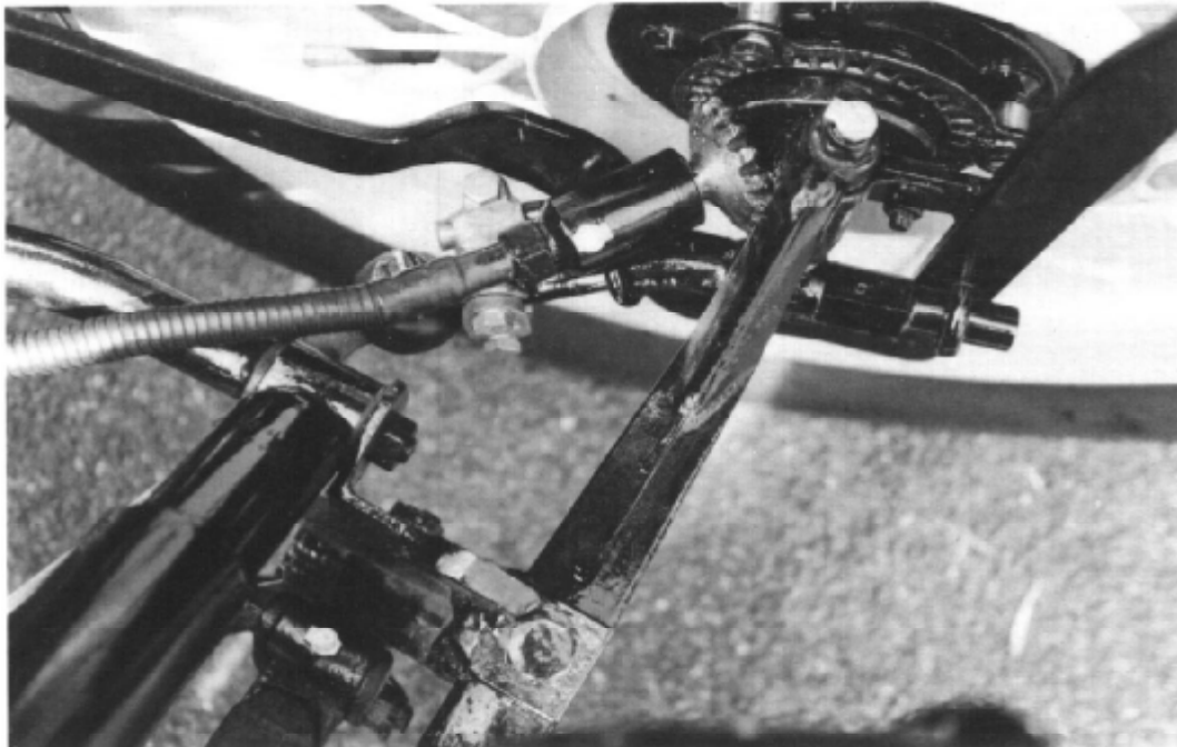
Above: front axle support bar [spring loaded], crankcase support and radius rod mounting. Below: Left-hand front axle mounting with speedometer drive and fender support.
