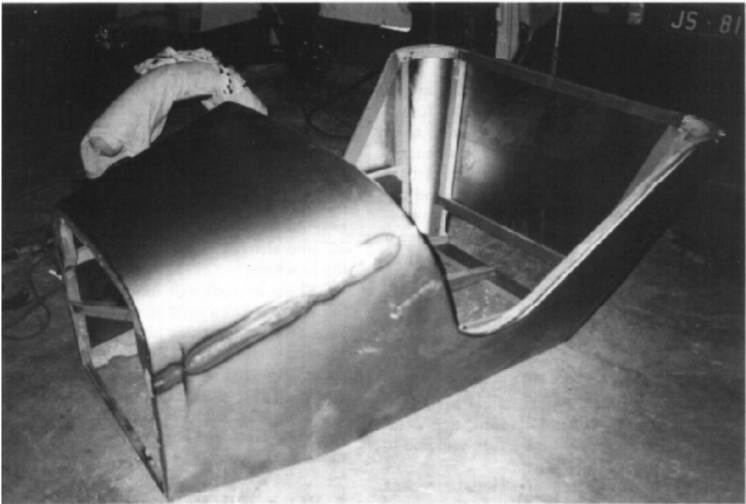
Above: Body skin being applied. Below: Body skin completed.
