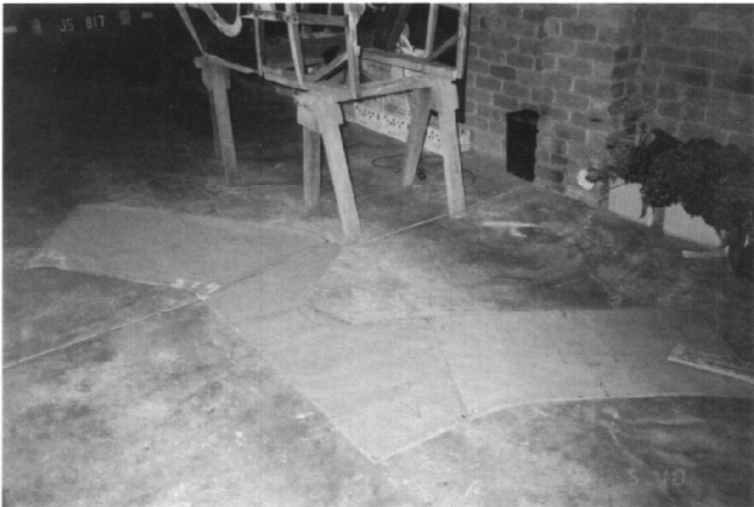
Above: Making paper patterns for body skin. Below : Final patterns are laid out on floor, ready for attaching to sheet metal and cutting to fit.
