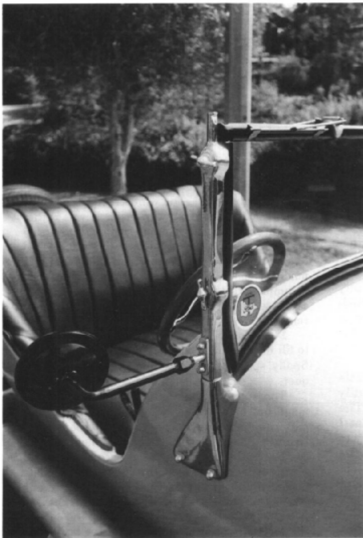
Windshield and details of its mounting to the body.
