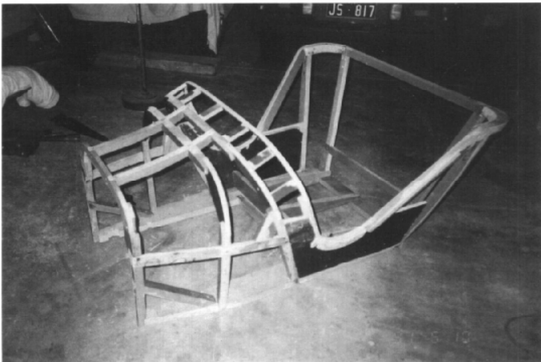
Below: Body woodwork is completed and ready for "skinning."
