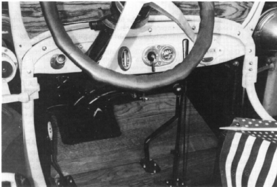
Above: Photo shows two emergency brake levers-one in its normal position and one aft of the Ruckstell shifter. In actuality, the lever in the normal position merely actuates "neutral." The lever in the center actuates the emergency brake.
