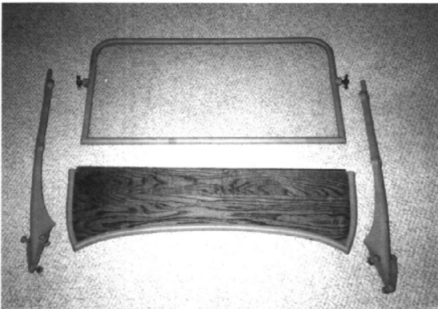
A stock Model T windshield was narrowed, shortened and general/y modified to fit the four-inch narrowed body
