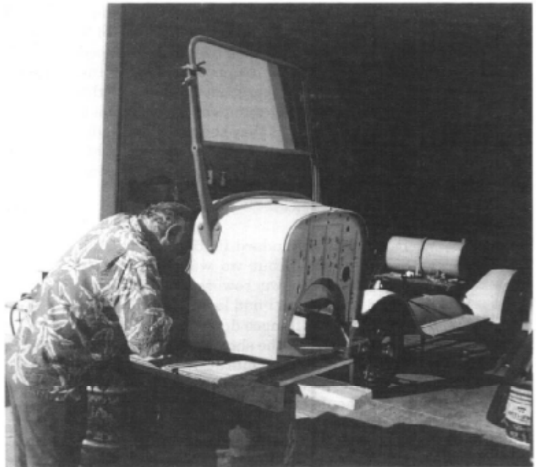
Jerry Fugit tries fitting another variation of a special emergency brake bracket
