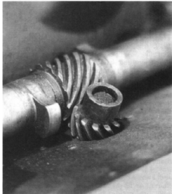
Close up of the cam lobe and distributor drive gears of the "Two Up & Two Down" Winfield engine.
