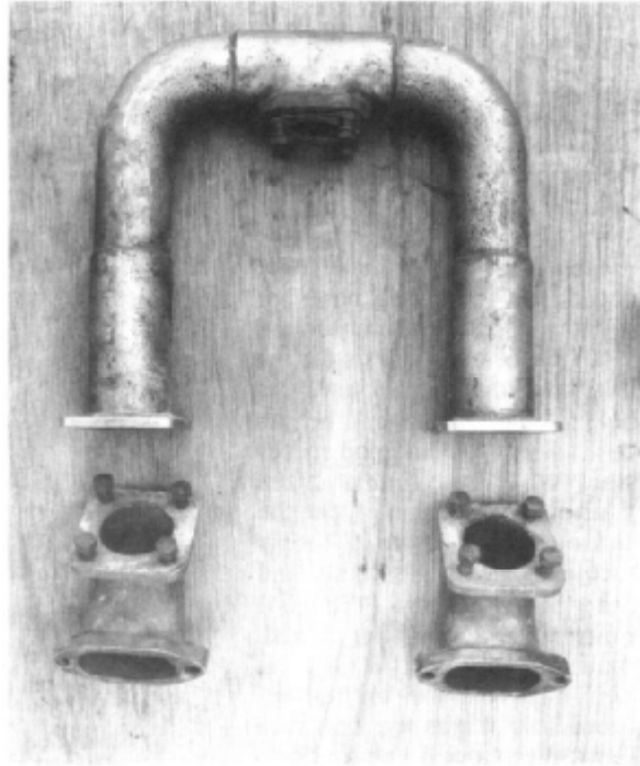
The intake manifold and adaptors used on the "Two Up & Two Down" engine. Ed Tate photo.
