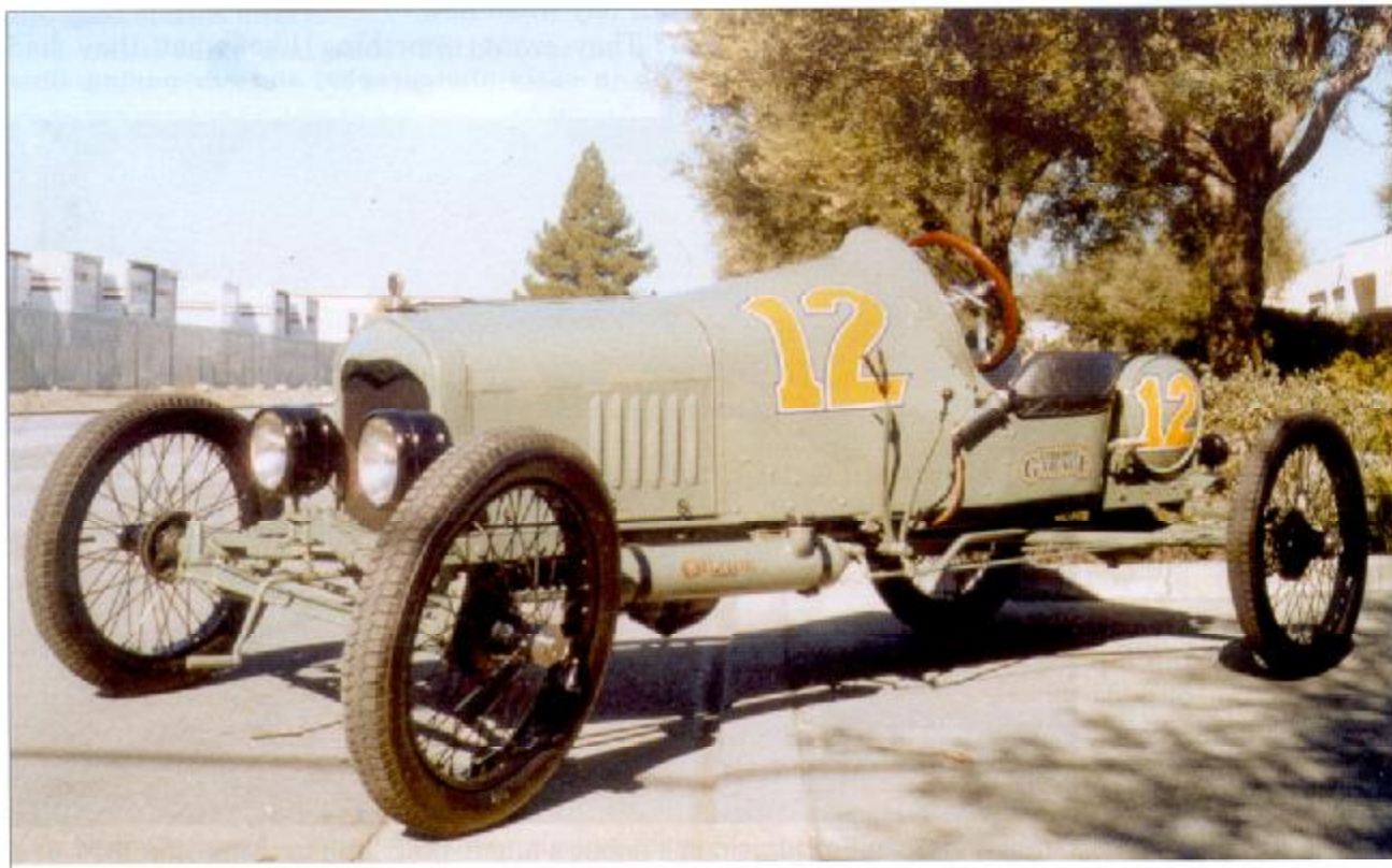
Lobuck—the next generation. Colin and Grant's deluxe creation. Lobuck no more. The Budd 30" x 31/2" wire wheels are the latest addition. Note the unique radiator shell and left side under-body auxiliary oil tank with the Oilzum logo.
